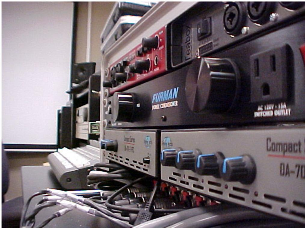
Figure 6.9: PLOrk rack: audio interface, amplifiers, power conditioner, Teabox.
